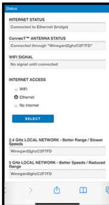
**\*NOTE:** Factory Reset is required to get the unit out of Bridge Mode. You will need to power on the unit, wait 90-150 seconds and then power off. Repeat 3 consecutive times. On the next power on, the system will begin a reset, this process could take up to 5 minutes.
