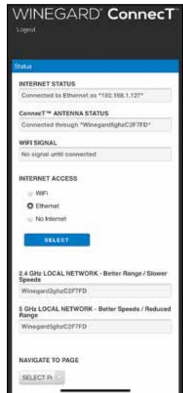
**Bridge Mode\*** – Allows passthrough of your home router connections. In this mode devices connected to the Extreme's SSIDs/network will get the same IP subnet as all other devices connected directly to your home router.
