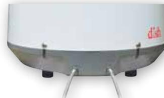
3. Tighten coax connections until fingertight, and then tighten a quarter turn more with a wrench. Do not overtighten.
