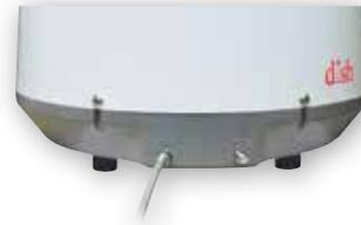
**NOTE** The receiver provides power to the electronics via the main port. There will be no power to the electronics if a coaxial cable is connected to the secondary port but not the main port.
