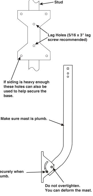
Tighten securely when mast is plumb.
